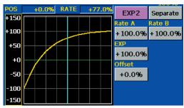
Using the EXP2 curve is helpful in engine rise and other engine control.
