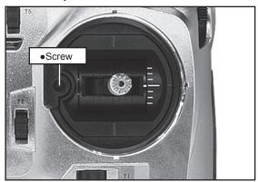
Use the attached 1.5mm hexagonal wrench (inside stylus) to turn the screw clockwise to adjust the stick outwards, or counter-clockwise to tilt it inward
