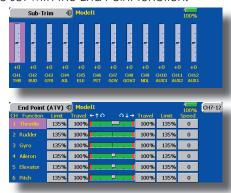
• Swash plate correction (Except H-1 mode) Operation of the swash plate near the hovering point can be corrected by swash AFR function correction mixing. Use this when pitch, aileron, and elevator operation causes the swash plate to deviate from the normal direction.
