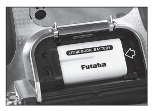
4. Close and lock the battery cover until you hear a snapping sound.
