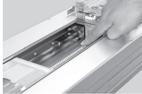
Applying grease to the linear guide Applying grease to the ball screw
