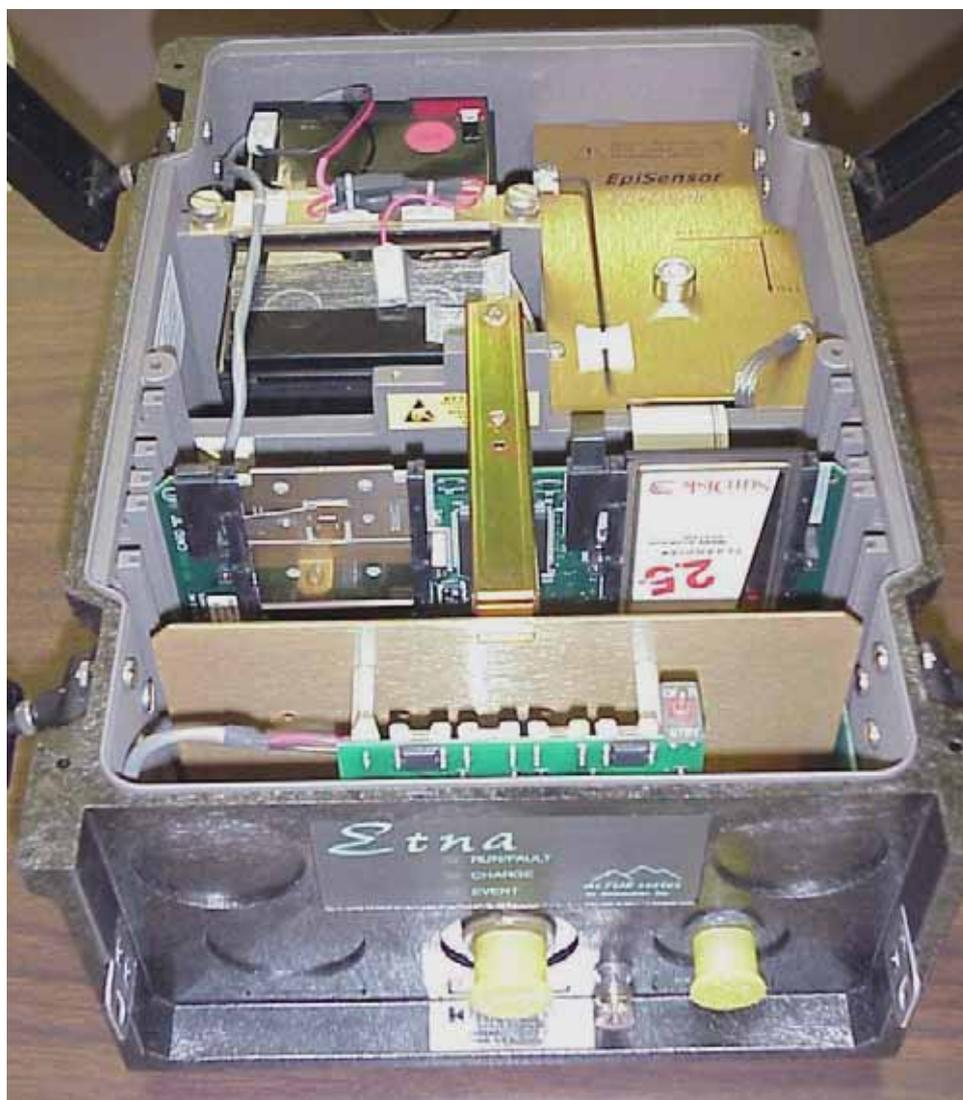
This Etna is equipped with the optional 12V, 12 Ah battery. 图中 Etna 配置有 12V,12Ah 电池选项。
