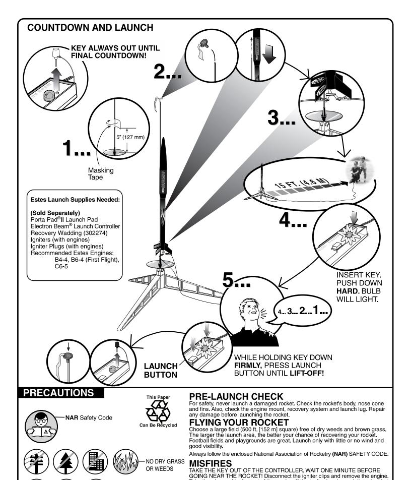
Take the plug and igniter out of the engine. If the igniter has burned, it worked but did not ignite the engine because it was not touching the propellant inside the engine. Put a new igniter all the way inside the engine without bending it. Push the
