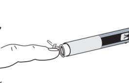
**F.** Insert engine into rocket.
