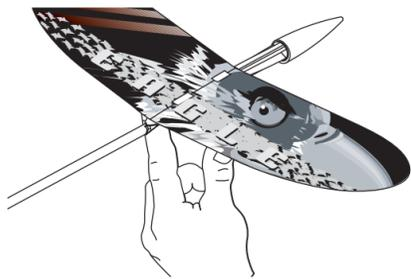
**B.** Add clay weight to the fuselage just behind the nose cone, until the glider balances at these points.
