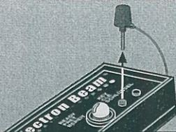
**9...** Remove the safety cap from the launch rod. Slide the rocket's launch lugs down the launch rod. Make sure rocket slides freely.
