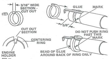
7 Cut a 3/16" wide section from one of the centering rings (part B). Place a mark on the engine tube 5/8" from end. Apply a bead of glue around tube in rear of mark. Don't get
