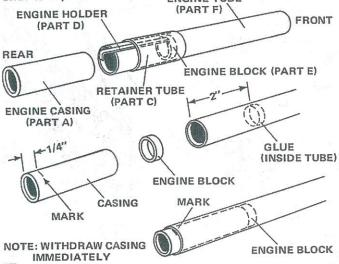
Locate the parts shown in the illustration. Place a mark on the engine casing 1/4" from one end. Using a small stick, apply a bead of glue inside one end of the engine tube approximately 2" from the end. Insert the engine block into this end of the tube and use the engine casing to push the block into place (with mark on casing even with end of engine tube). Withdraw casing immediately so it will not be accidentally glued into tube.
