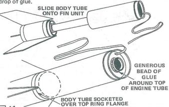
Slide the body tube assembly onto the fin unit. The bottom of the body tube should be socketed over the upper section of the fin ring and the engine tube should extend through the die-cut ring at the top of the body. Make sure the whole unit is pushed tightly together, then apply a generous bead of glue to the engine tube where it protrudes through the die-cut ring. Set the assembly aside and do not disturb until
