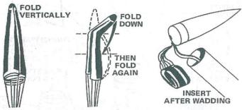
T-12 Loosely fold the parachute. Lay it on top of the wadding, with its shroud lines and shock cord on top of it. Slide the nose cone into place.
