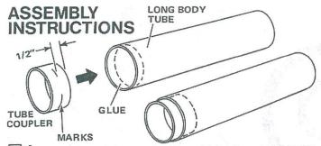
Mark the tube coupler (part L) in the middle (1/2" from one end). Put 3 or 4 marks around coupler so it can be positioned straight in the body tube. Run a bead of glue around the inside of one end of one 9" long body tube (part K). Push the coupler into the tube until the marks on the coupler line up with the end of the tube. Wipe away excess glue and set aside to dry.
