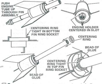
9 Slide the engine tube assembly up through the fin assembly as shown. Note that the engine holder must be centered
