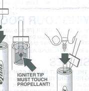
C. Insert igniter plug. Firmly push all the way in!
