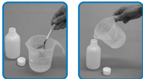
**NOTE:** After a while, the solution will change to a light brown color. This is normal and the solution can be used over again to generate 100's of launches! When not in use, pour solution back in bottle and save.
