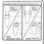
Parachute should slide easily into body tube. If fit is too tight, unfold and repack again.
