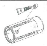
C. Cement a launch lug into the recessed area on engine mount as shown.
