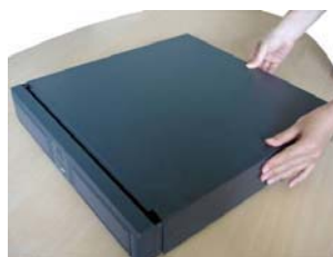
②拆下主机上盖
