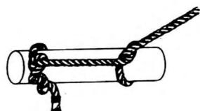
Figure 4:13 Timber Hitch and Half-Hitch for Lifting Spars
