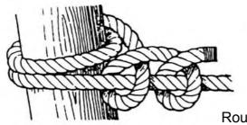
Figure 4.11 Round Turn and Two Half-Hitches
