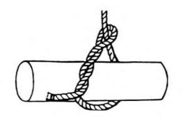
Figure 4:12 Timber Hitch
