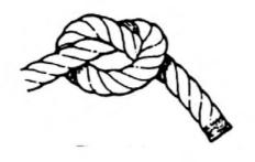
Figure 4:4 Thumb Knot
