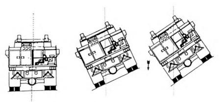
Figure 4:1 Vehicle Centre of Gravity
