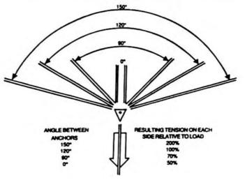
Figure 4:3 Relationship Between Sling Angles and Tension
