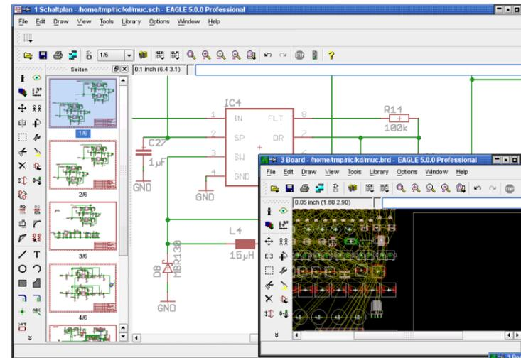
Now the desired connections (shown as rubber bands) are converted into non-crossing tracks. In EAGLE this can be done by hand, or the Autorouter can do it automatically. Critical connections are usually made by hand, while the remainder are left to the Autorouter.
