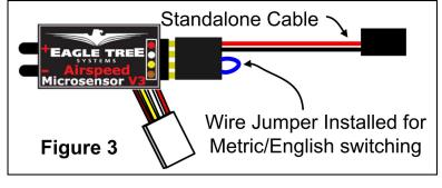
the wrong units are configured, just disconnect the power from the MicroSensor and reconnect it.
