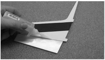
**2.**  $\Box$  Glue the rudder onto the fin using thin CA.
