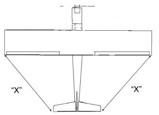
**4.** □ Measure from the end of the wing to the tip of the stab. This measurement should be the same for both sides.
