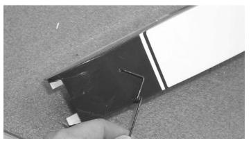
**3.**  $\Box$  Insert the nose gear wire through the hole in the bottom of the fuselage.
