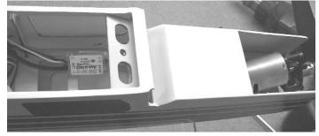
□ Insert the speed control and motor assembly through the front of the fuselage and into the main cabin of the fuselage.
