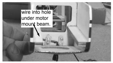
Place the nose gear wire in the center of each strap and insert the end into the far hole under the motor mount beam.
