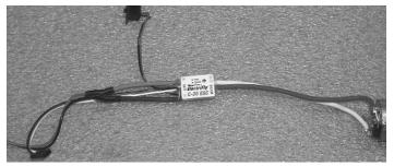
2. □ Solder your speed control onto the motor, by following the instructions that came with your speed controller.
