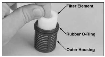
□ 3. Remove the air filter parts from the parts pack. Slide the large rubber O-ring around the threads of the outer housing. The O-ring will help seal the air filter housing together. Soak the air cleaner element with an air filter oil, light machine oil, or, in a pinch, shock oil. Thoroughly soak the foam element and squeeze out the excess. Then install the filter element into the plastic outer housing.
