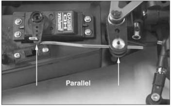
☐ 27. Remove the screw from the steering servo horn. Slide the steering linkage rod through the hole in the linkage rod connector in the steering arm. Place the servo horn back onto the servo. When placing the horn onto the servo, the horn and the steering arm should be parallel as shown in the photo. Note: Do not screw the servo horn down yet, the servos will need to be centered after assembly is completed.
