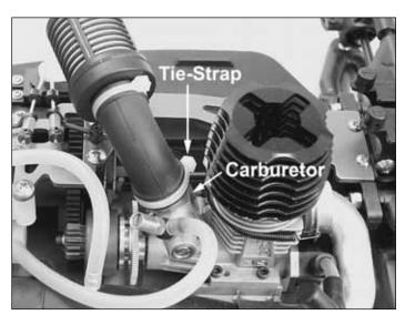
☐ 44. Place the air filter onto the carburetor. Using the remaining included tie-strap, tightly secure the air filter to the carburetor. Cut the excess portion of the tiestrap off to avoid interference.
