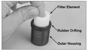
☐ 40. Assemble the air filter. Slide the large rubber O-ring around the threads of the outer housing. The O-ring will help seal the air filter housing together.
