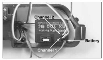
☐ 15. Plug the steering servo, throttle servo and switch into the receiver. See your radio instructions to determine which channel is steering and which is throttle. Plug the switch into the battery socket.
