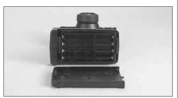
□ 9.Slide open the battery door on the bottom of the transmitter. Place 8 "AA" batteries into the holder in the configuration molded into the plastic on the battery holder. Re-install the battery door.
