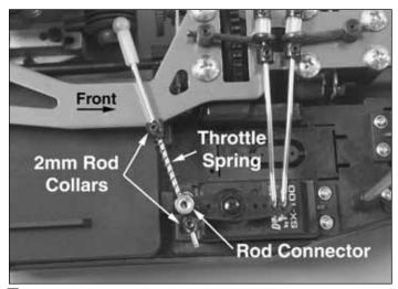
☐ 47. With the throttle servo still in neutral, push the throttle rod so that the carb closes. Move the rod collar against the rod connector and tighten the set screw. Move the other rod collar so that the throttle spring is *slightly* compressed and tighten the set screw.
