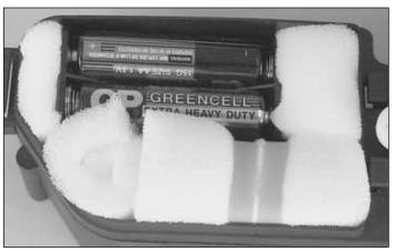
□ 20. Cut the left over foam into small pieces and place them around the receiver and battery to help secure them into place. Then slide the radio box cover back onto the radio box.
