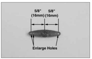
□ 29. Remove the servo horn from the throttle servo. Using a 5/64" (2mm) drill bit or hobby knife, enlarge the two farthest holes at one end of the servo horn and the farthest hole on the other end.
