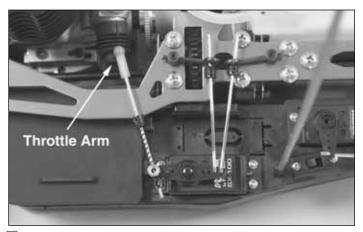
☐ 35. Snap the ball cup onto the throttle arm on the carburetor. Install a second rod collar onto the throttle linkage so that it fits against the rod connector. **Note:** Do not tighten the set screw in the rod collar, the linkage will be adjusted later.
