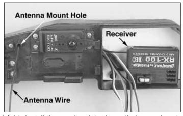
☐ 14. Install the receiver into the radio box and route the antenna wire through the same hole the servo leads come in. Run the antenna wire up through the antenna mount hole.
