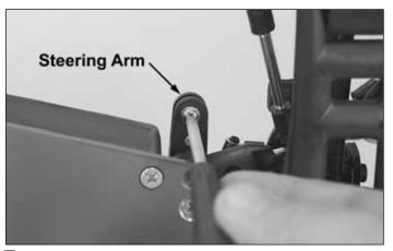
☐ 26. Loosen the screw in the bottom of the steering arm on the servo saver enough for the linkage rod to slide through the metal rod connector.
