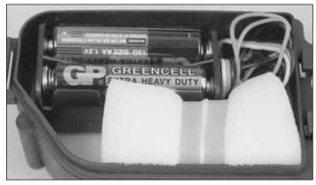
☐ 19. Install the receiver into the receiver box as shown. Make sure all of the wires are out from under the receiver so that it will properly fit into the radio box.
