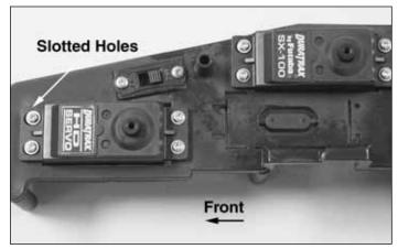
■ 8. Mount the servo to the radio tray using four mounting screws included with the radio system. Use the other mounting block that you cut out of the radio tray in step 4 and place it against the under side of the radio tray under the slotted holes. The screws should go through the servo, the radio tray and into the servo mounting block. Note: Make sure to use the mounting block on the end with the slotted mounting holes.
