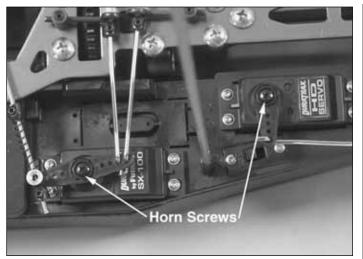
□ 48. With the transmitter and receiver still on, remove the steering servo horn. While the front wheels are positioned straight, re-install the steering servo horn, so that the wheels remain as straight as possible. The fronts of the wheels may be slightly inward (that's O.K., this is called "toe-in", see page 17.)
