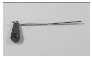
☐ 25. Install the z-bend end of the linkage rod into the servo horn from the bottom as shown.
