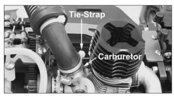
□ 5. Place the air filter onto the carburetor. Using the remaining included tie-strap, tightly secure the air filter to the carburetor. Cut the excess portion of the tiestrap off to avoid interference.
