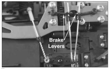
☐ 33. Re-install the servo horn onto the servo. Slide the brake linkage rods through the brake levers as shown.
