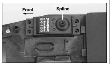
☐ 5. Place the standard throttle servo into the radio tray. **Note: Notice the direction of the servo spline when installing.** Run the servo lead into the radio box through the hole in the side.
