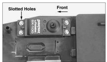
G. Mount the servo to the radio tray using four mounting screws included with the radio system. Use one of the servo mounting blocks that you cut out of the radio tray in step 4 and place it against the under side of the radio tray under the slotted holes. The screws should go through the servo, the radio tray and thread into the servo mounting block. Note: Make sure to use the servo mounting block on the end with the slotted mounting holes.
