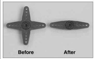
□ 9. Cut two of the arms off the throttle servo horn by scoring both sides of the arm with a hobby knife and snapping off the arms with pliers.
