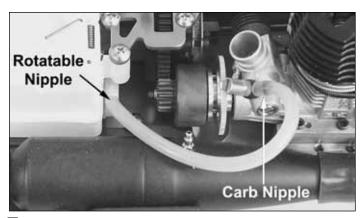
□ 38.Install one end of the 6" (150mm) piece of fuel tubing onto the rotatable nipple on the rear of the fuel tank and the other end onto the nipple on the carburetor.
