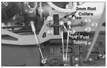
☐ 36. Slide a 1/4" piece of fuel tubing over each of the brake linkage rods. Then install a rod collar onto each of the two rods. Note: Do not tighten the set screw in the rod collars, the linkage will be adjusted later.
