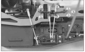
□ 34. Screw the plastic ball cup onto the throttle linkage wire. Install one rod collar onto the linkage rod, then slide on the throttle linkage spring. Insert the throttle linkage through the rod connector as shown. Note: Do not tighten the set screw in the rod collar down, adjustments will be made later.
