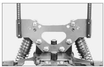
☐ 11. Remove the lower screw from each of the body posts so that the posts can be placed upright. Reinstall the screw through the shock tower into the body post as shown.
