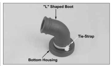
☐ 4. Press the "L" shaped boot onto the bottom housing of the air filter. Using one of the included tie-straps, tightly secure the boot onto the bottom housing. Cut off the excess portion of the tie-strap. Screw the bottom and outer filter housing together. **Note: Overtightening will strip the threads.**
