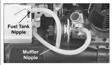
□ 39.Install one end of the 4" (100mm) piece of fuel tubing onto the nipple next to the fuel tank lid and the other end on the nipple on the muffler.
