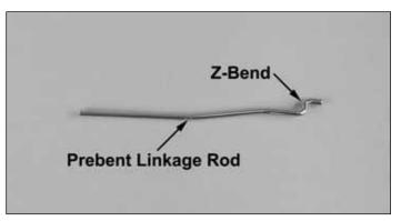
☐ 23. Remove one of the three pre-bent linkage rods with a z-bend at the end of it from the linkage bag. Note all of the pre-bent rods are the same.
