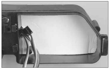
☐ 13. Route the wires and connectors for the switch and two servos through the hole in the radio box. Cut a piece of foam the size of the radio box and place it in the bottom for all of the equipment to set on. Make sure that all of the wires coming into the radio box are on top of the foam. This is to help prevent vibration damage to the receiver.
