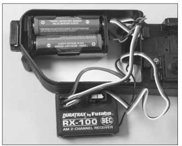
☐ 17. Install the receiver battery into the radio box. Note the placement of the receiver battery in the box. Connect the receiver battery to the remaining end of the on/off switch.
