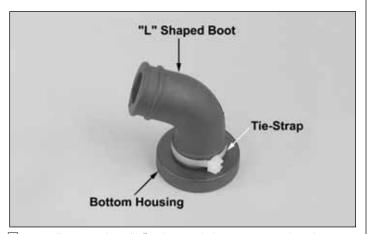
☐ 42. Press the "L" shaped boot onto the bottom housing of the air filter. Using one of the included tiestraps, secure the boot tightly onto the bottom housing. Cut the excess portion of the tie-strap to avoid interference.
