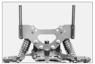
☐ 49. Remove the lower screw from each of the body posts so that the posts can be placed upright. Reinstall the screw through the shock tower into the body post as shown. The height of the body can be adjusted by raising or lowering the posts on the shock tower.
