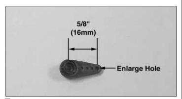
☐ 24. Remove the servo horn from steering servo. Using a 5/64" (2mm) drill bit or hobby knife, enlarge the hole 5/8" (16mm) away from the center of the horn.
