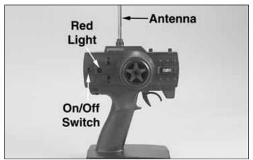
■ 8. Remove the transmitter antenna from the holder and screw it into the hole on the top of the transmitter.
