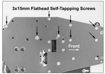
☐ 2. Remove the radio tray from the chassis by removing the (8) 3x15mm flat head self tapping screws from the bottom of the chassis.
