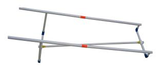
There will be four sections with a blue 90 degree connector on them. these are the upright sections the two long pieces should be at the front of the mount and the short ones at the back. The two orange pieces slide together and mount to the uprights with the longer dowels inserted into the taller uprights.
