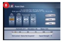
Input **zip code of current location** and dish type. Zip Code should be the zip code of **your current location**. Note that whenever you move the satellite antenna to a new **location**, you must enter the zip code of your new current location.
