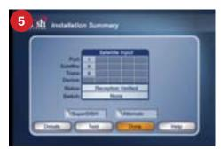
Select **Test**. It will go through a number of steps, then return to the screen shown here with previous information cleared. If at any point it asks you to save, select **Save** or **Yes**. Select **Done**. Reconnect the coaxial cable to the "Sat In" port on back of receiver. Now **turn on** the antenna. Allow it 3–4 minutes to acquire satellites.
