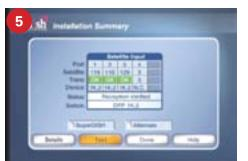
Check that there are no checkmarks by SuperDISH or Alternate. Select **Test**.
