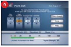
Once accurately pointed, the signal meter will turn green. Make small adjustments to get the signal as high as possible. Check that the bar at the bottom of
