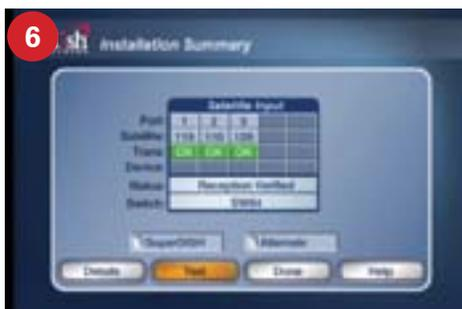
6 Check that there are no checkmarks by SuperDISH or Alternate. Next, select **Test** again. This time it will install the SW64 switch. *This SW64 switch is a DISH Network receiver setting, not a physical part.* If the SW64 switch is not obtained, run the Check Switch test again.
