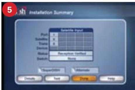
5 Select **Test**. It will go through a number of steps, then return to the screen shown here with previous information cleared. If at any point it asks you to save, select **Save** or **Yes**. Select **Done**. Reconnect the coaxial cable to the "Sat In" port on back of receiver. Now **turn on** the antenna. Allow it 3–4 minutes to acquire satellites.
