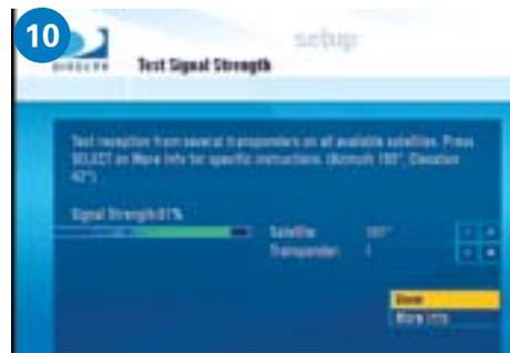
**Once accurately pointed**, the signal meter will show a signal strength. You'll want to make small adjustments to **get the signal as high as possible**. Once the signal is peaked, select **Done**.
