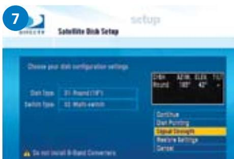
7 In the box, it now gives you an **AZIM** (Azimuth Angle) and **ELEV** (Elevation Angle). These are the pointing angles you will need when you go to point the dish. Now select
