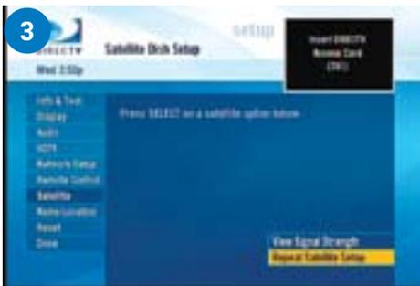
3 In your receiver Menu, you will need to identify the Satellite Menu. The Satellite Menu will have an option for **Satellite Setup**.
