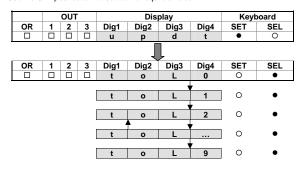
The "FAIL" text alternated with "Hi" or "Lo" is visualised if the detection is not correct. Repeat the procedure starting from the operating mode
