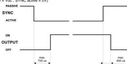
A typical application of the SYNC function is the necessity to detect a particular position in a multicoloured target while the other area must not be detected. This function can also be used to avoid erroneous detection during target-background transitions.
