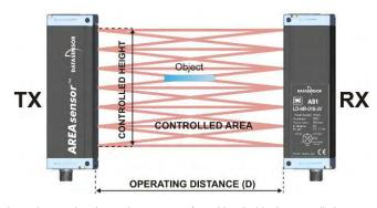
The beam interruption due to the passage of an object inside the controlled area causes the closing of the switching output and the variation of the device analogue output signal. Small objects can be detected (reaching dimensions of only 0.5 mm) and with a reduced
