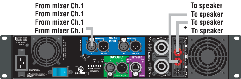
Figure 4 Rear Panel Connections for Bridge-Mono Wiring
