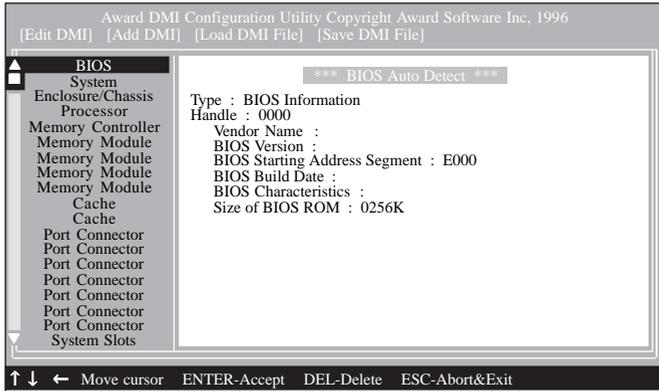
The four menus located on top of the DMI Configuration Utility screen are Edit DMI, Add DMI, Load DMI File and Save DMI File. Use the ← or → (left or right) arrow keys to select a menu from the Menu bar.
