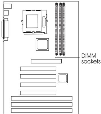
The system board is equipped with three 168-pin DIMM (Dual In-line Memory Module) sockets that support x64/x72 unbuffered PC SDRAM DIMM, 3.3V.
