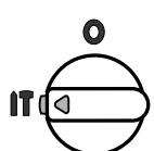
Position for **hammer drilling**
