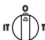
**Vario-Lock** position for adjustment of the chiseling position
