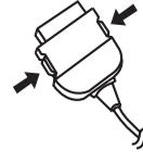
Pinch the lock buttons on both sides of the connector and pull out.
