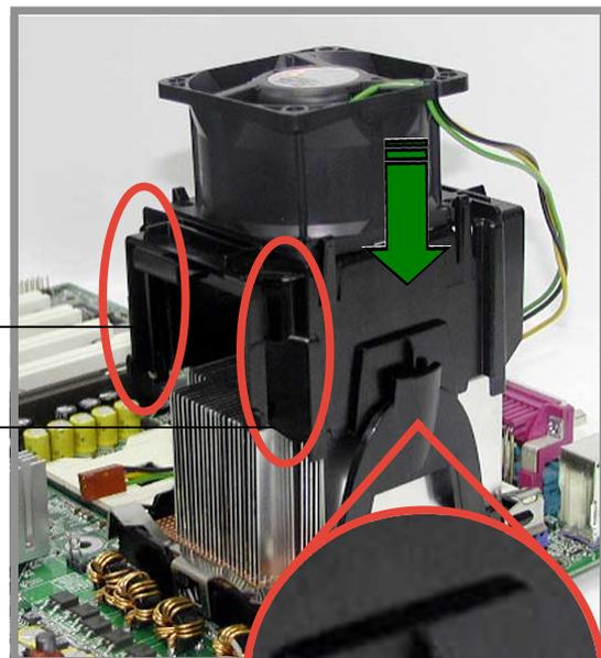
10. Align and insert the side rails of the air tunnel into the grooves on the retention mechanism.
