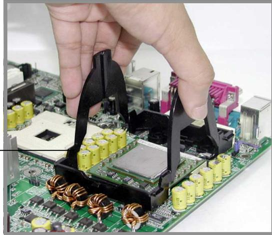
3. Secure the retention mechanism with the thermal plate using four screws.
