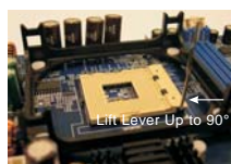
STEP 1: Lift The Socket Lever Up to 90°
