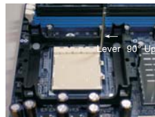
STEP 1: Lift Up The Socket Lever
