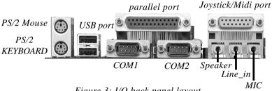
Figure 3: I/O back panel layout
