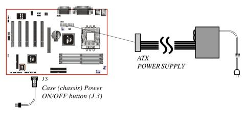
Figure 4: Simple ATX Power ON/OFF Controller
