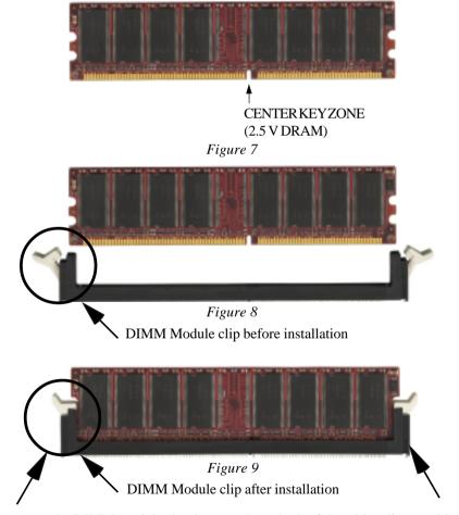
To remove the DIMM module simply press down both of the white clips on either side and the module will be released from the socket.
