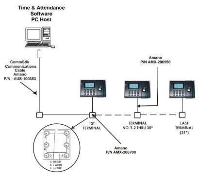
Figure 1-4 Multiple Direct Connect Serial Terminals
