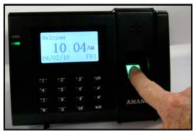
Figure 2-1 Punching Using Biometrics
