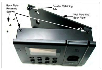
Figure 1-2 Back Plate For Wall Mounting
