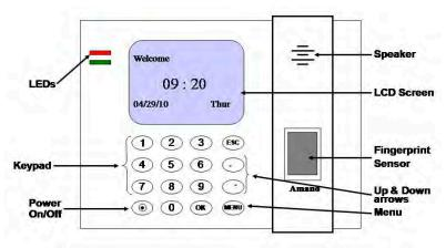
Figure 1-1 FPT-40 Fingerprint Terminal Front View
