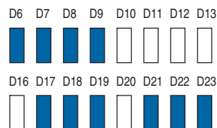
Figure 4-13. Condition of LEDs for Transmitting 3G-SDI Level A Video Standard
