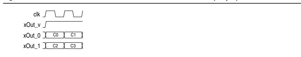
Figure 4-19. Four Channels on Four Wires with Double Clock Rate (Output)
