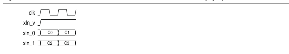
Figure 4-18. Four Channels on Four Wires with Double Clock Rate (Input)
