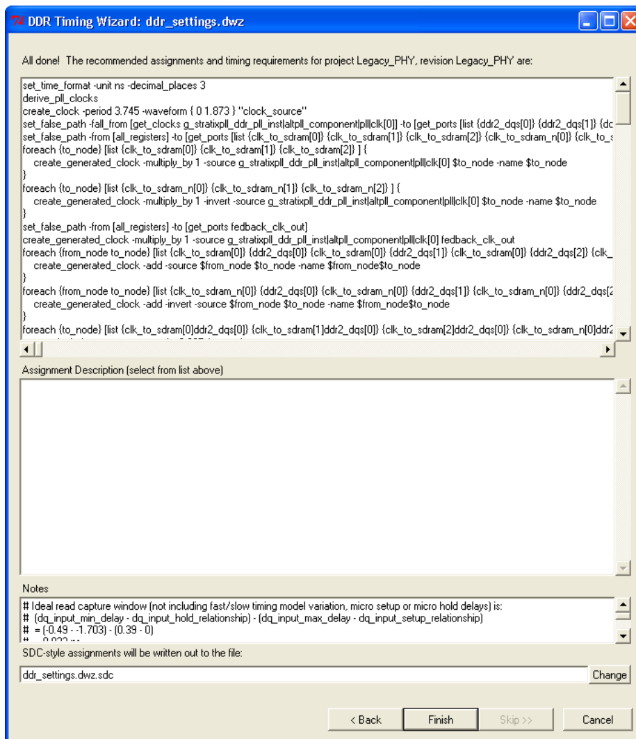
Figure 2–31. Last Page of the DTW When Using TimeQuest Timing Analyzer
