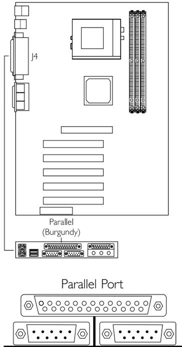
The system board has a standard parallel port (J4 - Burgundy) located at the ATX double deck ports of the board for interfacing your PC to a parallel printer. It supports Normal, ECP and EPP modes. You can set the port's mode in the Integrated Peripherals submenu of the BIOS.
