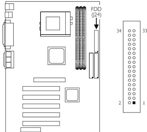
The system board is equipped with a shrouded floppy disk drive connector that supports two standard floppy disk drives. To prevent improper floppy cable installation, the shrouded floppy disk header has a keying mechanism. The 34-pin connector on the floppy cable can be placed into the header only if pin 1 of the connector is aligned with pin 1 of the header. You may enable or disable this function in the Integrated Peripherals submenu of the BIOS.
