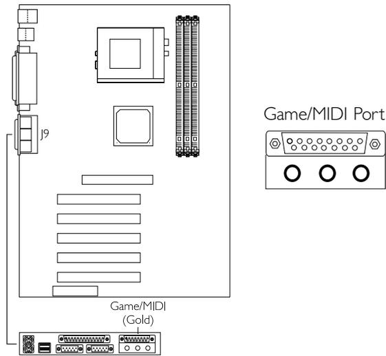
The Game/MIDI port is identical to that of a standard PC game adapter or game I/O port. Connect an analog joystick to the 15-pin D-sub connector (J9 - Gold) located at the ATX double deck ports of the system board. This port works well with any application that is compatible with the standard PC joystick.
