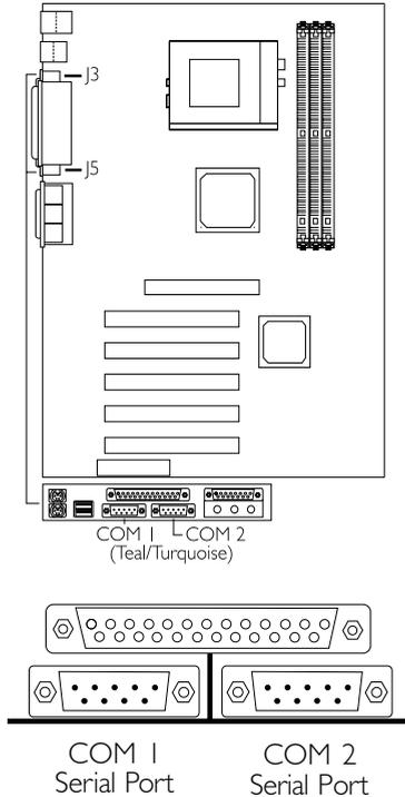
The system board is equipped with onboard serial ports (COM 1: J3 and COM 2: J5) - both in Teal/Turquoise color located at the ATX double deck ports of the board.
