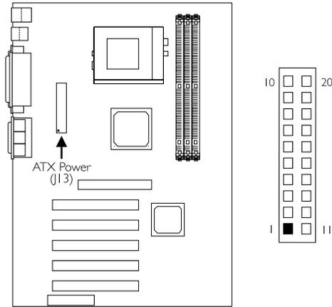
The pin assignment of the ATX power connector is shown below.
