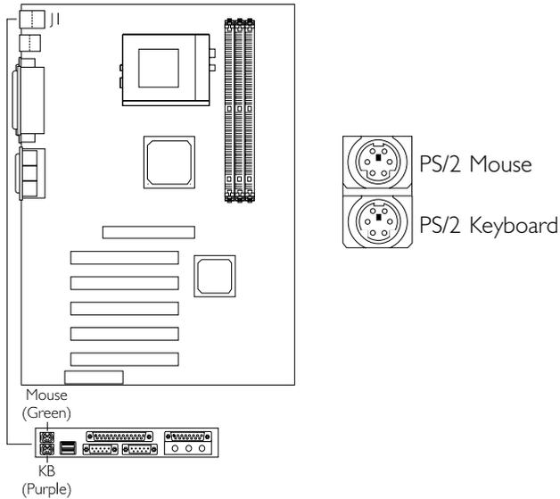
The system board is equipped with an onboard PS/2 mouse (Green) and PS/2 keyboard (Purple) ports - both at location J1 of the ATX double deck ports of the system board. The PS/2 mouse port uses IRQ12. If a mouse is not connected to this port, the system will reserve IRQ12 for other expansion cards.
