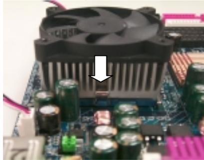
5. Hook one end of the cooler bracket to the CPU socket.
