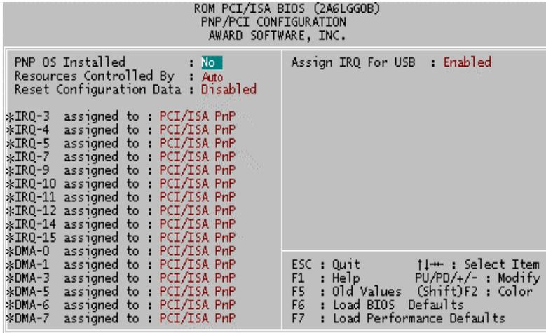
Figure 4.6: PNP/PCI Configuration
