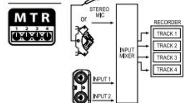
You can record tracks in MONO or STEREO from INPUT [1], INPUT [2] or the internal microphones. You can combine them with tracks recorded in other modes or <OVERDUB> additional tracks. In MTR mode, project data and settings are saved as a PROJECT in the MTR folder.
