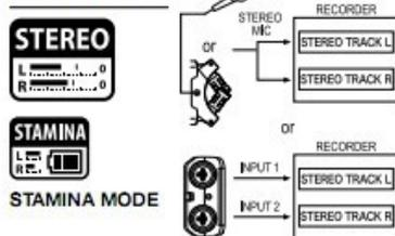
In STEREO mode, you can select 2 different inputs either INPUT[MIC] or INPUT[1] and INPUT[2], and operate them as one stereo file. The resulting FILE is saved in one of the ten sub-folders of the STEREO folder.
