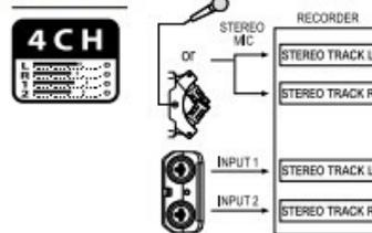
In 4CH MODE the H4n records two stereo WAV files: one stereo WAV file for the built-in microphones and one stereo WAV file for the inputs. These FILES are saved in one of the ten fixed folders.
