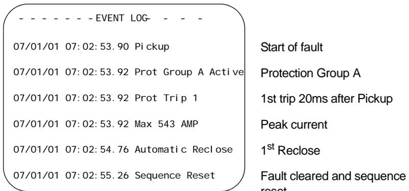
Figure 23: Sequence Reset Example
