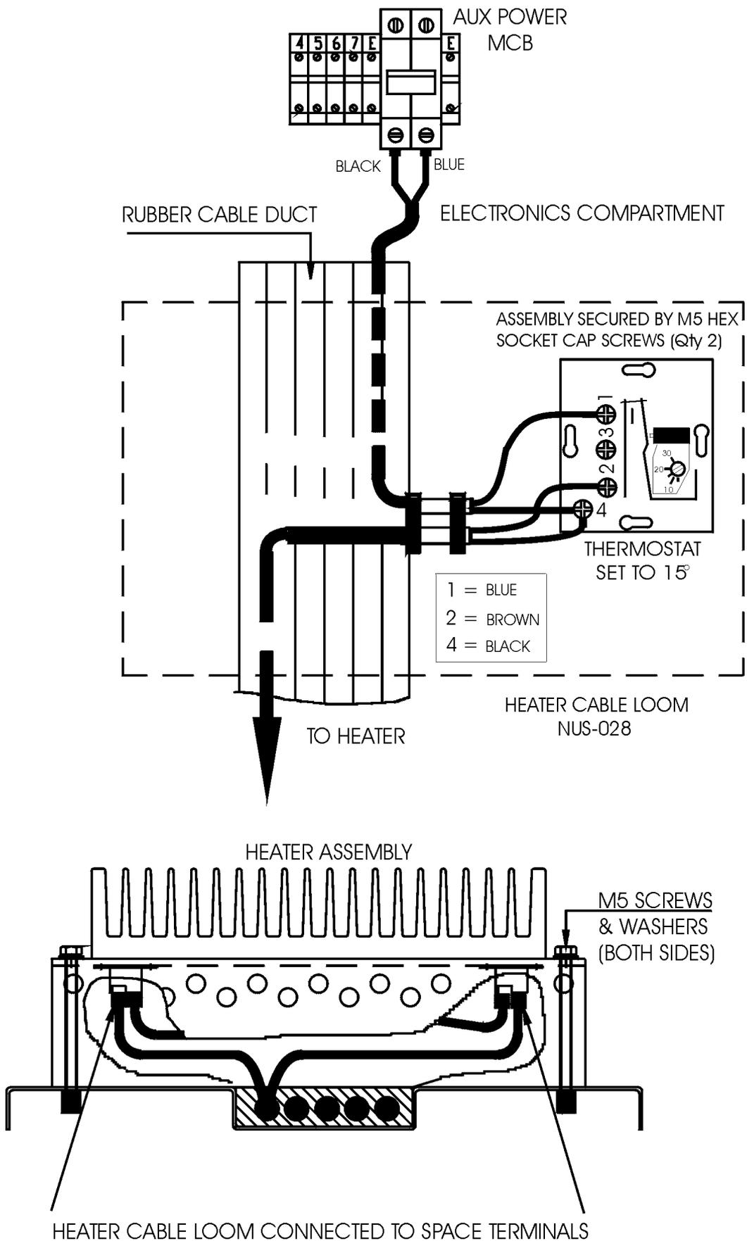
Figure 41: Control cubicle - Heater/thermostat connection
