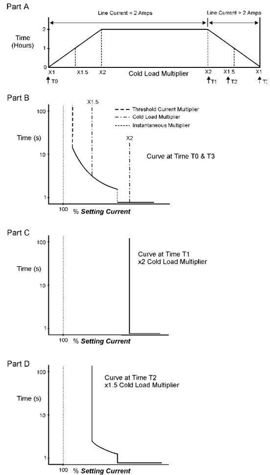
Figure 21: Cold Load multiplier (CLM) settings applied to protection curves
