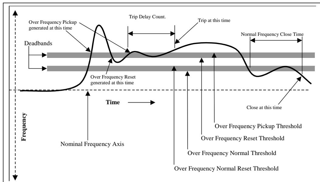
Figure 19: Over Frequency Detection
