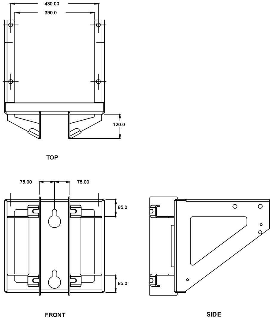
Figure 44: End Mounting Bracket
