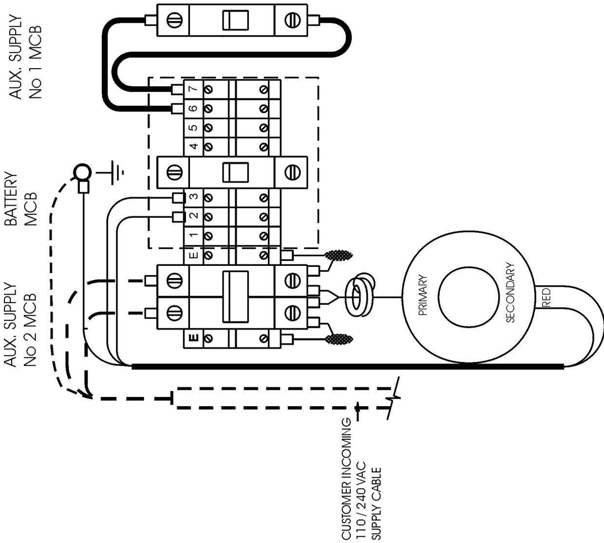
Figure 38: Control cubicle - Integrated plus LV aux power supply
