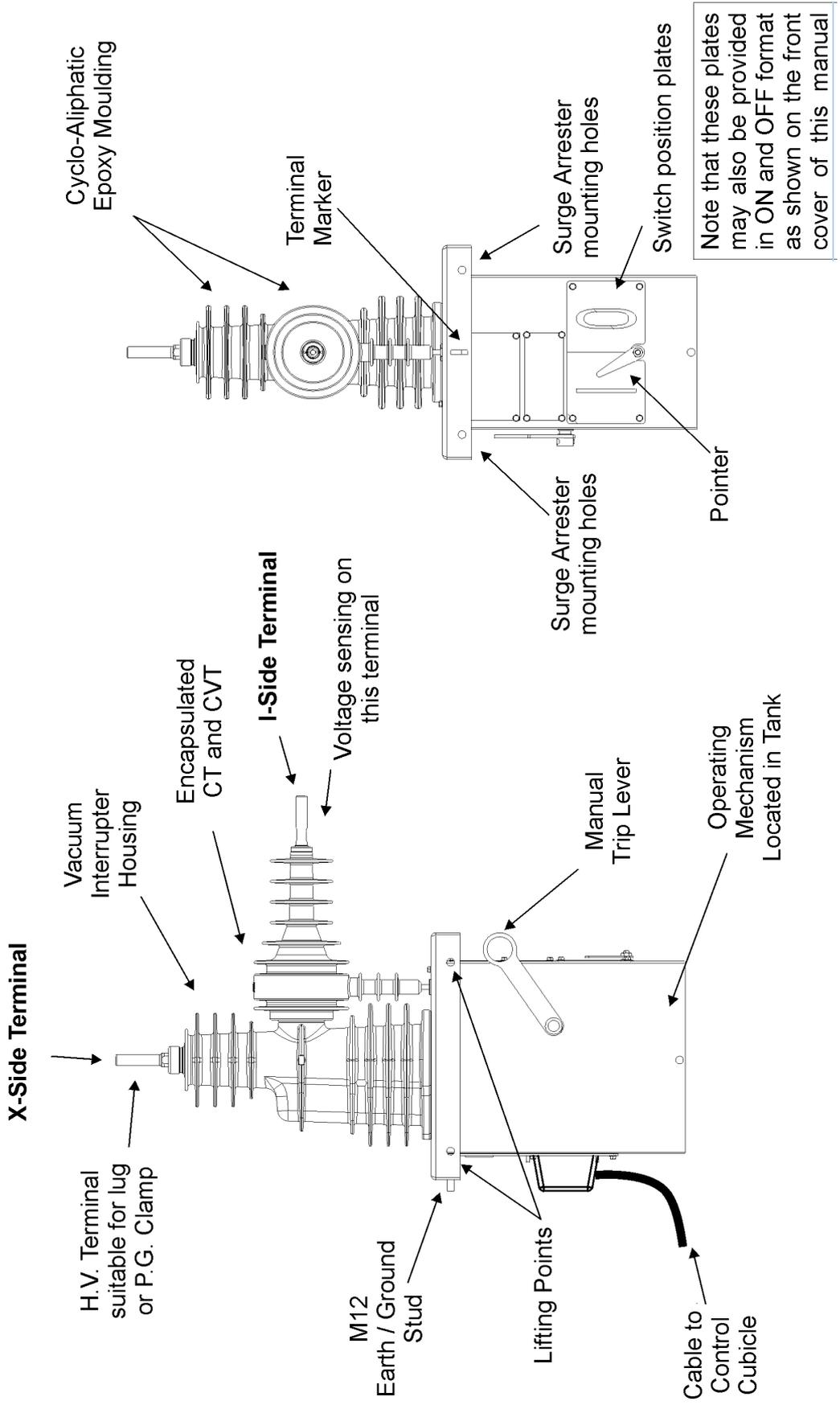
Figure 1: Circuit Breaker Features
