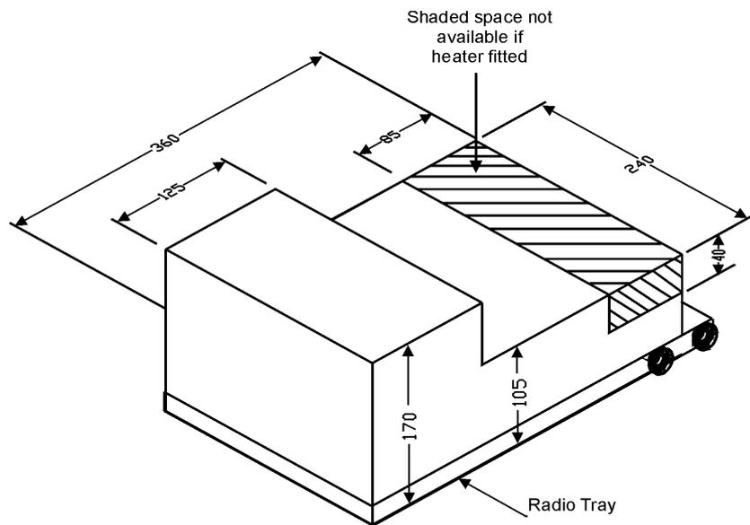
Figure 45: Radio mounting space
