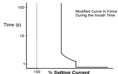
Figure 20: Effect of inrush current settings on a protection curve
