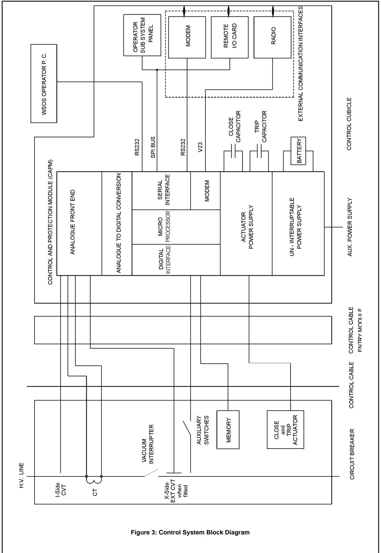
Figure 3: Control System Block Diagram
