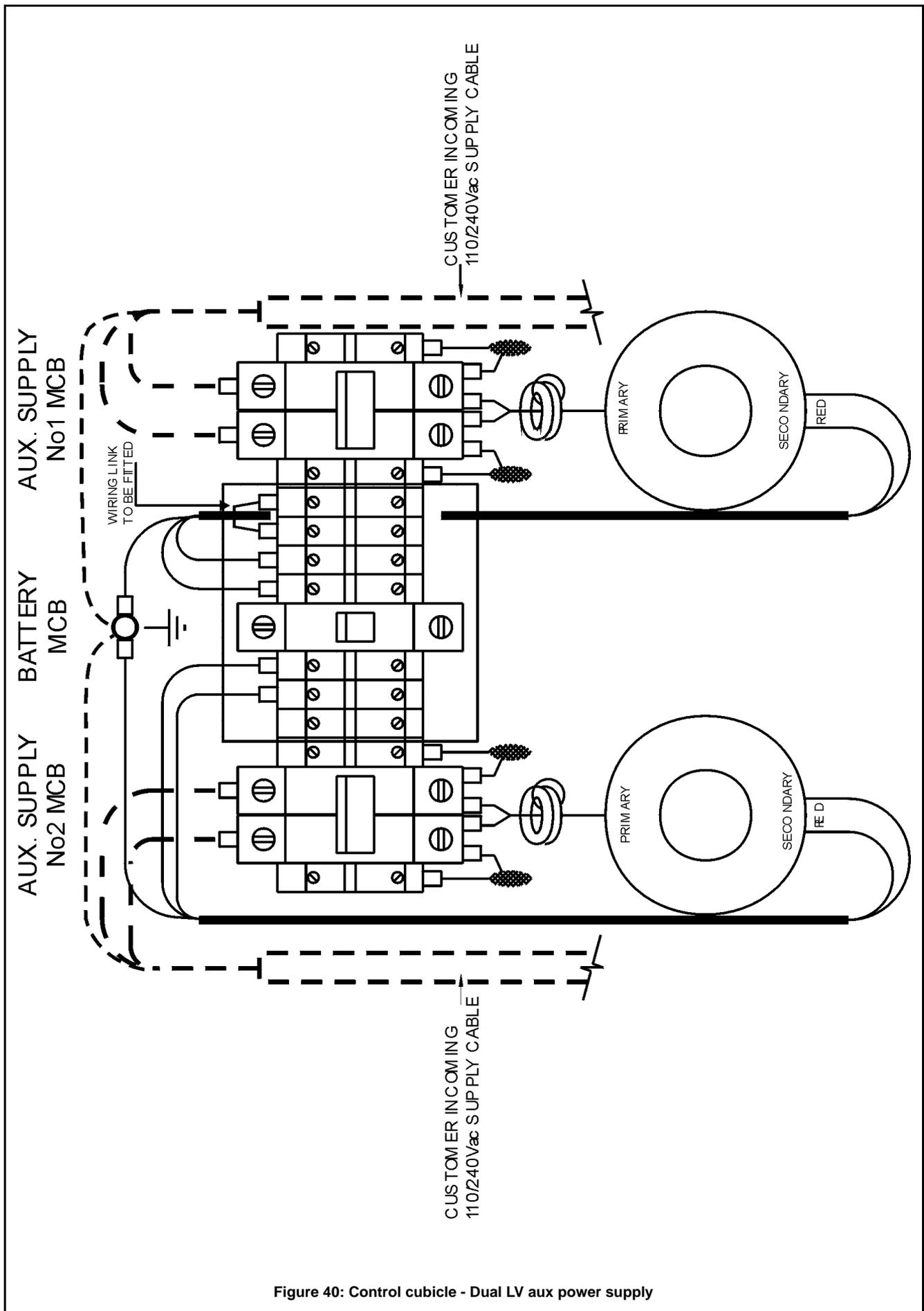
Figure 40: Control cubicle - Dual LV aux power supply
