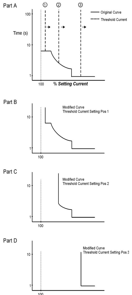
Figure 18: Composite curve changes due to different settings of threshold current multiplier
