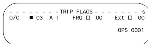
The counter next to the status indicator shows the number of times each protection element has caused a trip. Each counter has a range of 00 to 99 (cannot count past 99).
