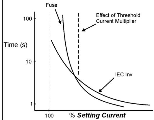
Figure 17: Co-ordination between fuse and IEC 255 inverse curve using the threshold current multiplier
