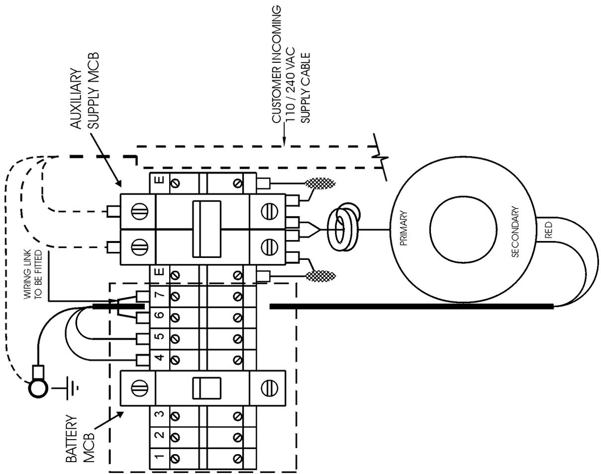
Figure 37: Control cubicle - Single LV aux power supply
