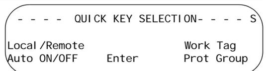
To configure a Quick Key press **SELECT** or **ENTER** and the following screen is displayed with the first field flashing.
