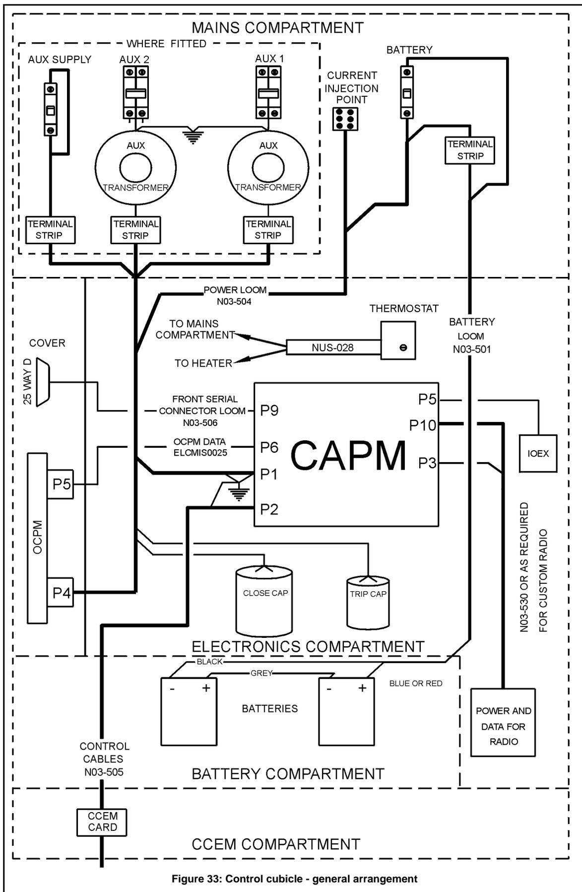
Figure 33: Control cubicle - general arrangement
