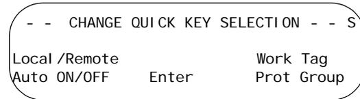
Pressing the **ARROW** keys will scroll the operator through the available functions. See Figure 5 (page 29).
