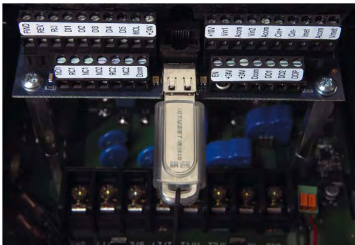
Figure 9: Vacon 500x Control Terminals
