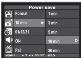
**4 Press the ▲ or ▼ key so that the desired time for the auto power off function is highlighted.**
