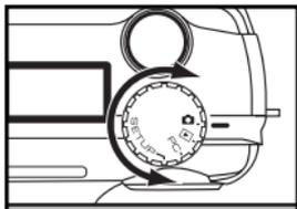
**2 Rotate the function dial to "SETUP".**
