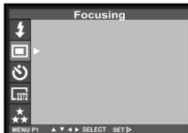
**2 Press the ▲ or ▼ key so that [FOCUSING] is highlighted and press the ► key.**
