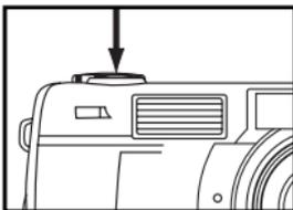
**7 Press the shutter-release button part-way down.**
