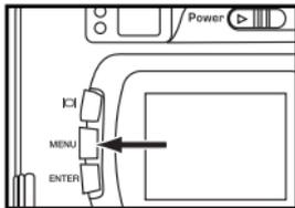
**1 Rotate the function dial to
