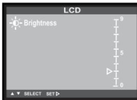
**3 Press the ▲ or ▼ key so that the desired brightness is highlighted, press the ► key to finish the setting.**
