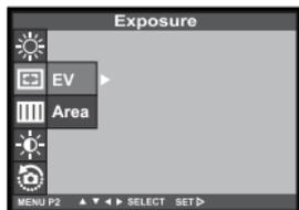
**3 Press the ▲ or ▼ key so that [EV] is highlighted and press the ► key press.**
