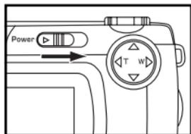
**1 When replacing the batteries, slide the power switch to turn off the camera.**
