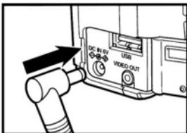
**1 Connect the mini plug of the DC adapter to the DC terminal of the camera.**
