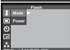
**3 Press the ▲ or ▼ key so that [MODE] is highlighted and press the ► key.**
