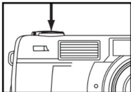
**4 Press the shutter-release button part-way down.**
