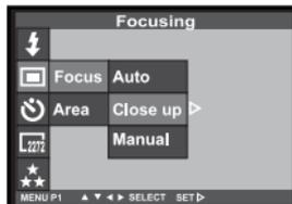
**4 Press the ▲ or ▼ key so that [CLOSE UP] is highlighted and press the ► key to finish the setting.**
