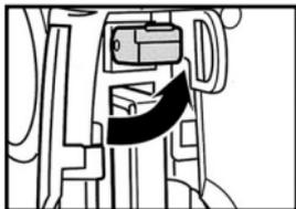
**3 Lift the card-release lever up as shown in the figure.**
