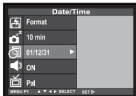
**6 Press the ▲ or ▼ key so that [DATE/TIME] is highlighted and press the ► key.**
