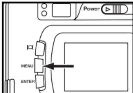
**1 After fixing the camera on the tripod, rotate the function dial to
