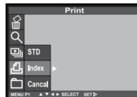
**3 Press the ▼ key so that [INDEX] is highlighted and press
