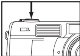
**5 Press the shutter-release button all-the-way down to take a picture.**
