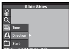
**6** Press the ▲ or ▼ key so that [DIRECTION] is highlighted and press ► key.
