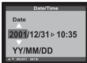
**5 Press the ▲ or ▼ key to specify or correct the date and press ► key to finish the setting.**
