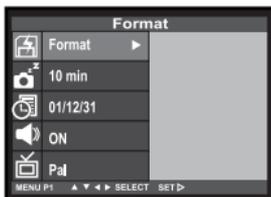
**3 Press the ▲ or ▼ key so that [FORMAT] is highlighted press ► key.**
