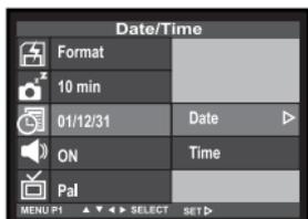
**4 Press the ▲ or ▼ key so that [DATE] is highlighted and press the ► key.**
