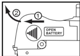
**2 Slide the battery-chamber door slightly in the ① direction and open it in the ② direction.**
