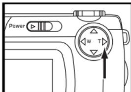
**1 In the recording mode, press the ► key in the recording mode so that the image is zoomed to the maximum.**
