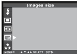
**2 Press the ▲ or ▼ key so that [IMAGE SIZE] is highlighted and press the ► key.**
