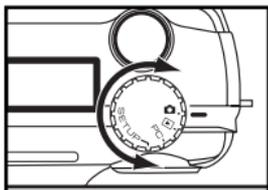
**2 Rotate the function dial to "SETUP".**
