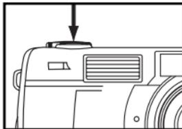
**6 Press the shutter-release button all-the-way down to take picture.**
