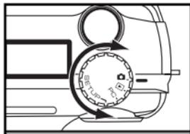
**2 Rotate the function dial to "SETUP".**
