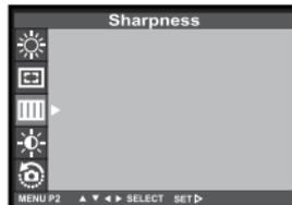
**2 Press the ▲ or ▼ key so that [SHARPNESS] is highlighted and press the ▶ key.**
