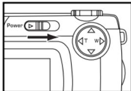
**1 Rotate the function dial to
