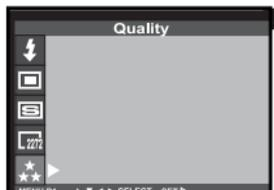
Press the ▲ or ▼ key so that the desired image size mode is highlighted press the ► key.
