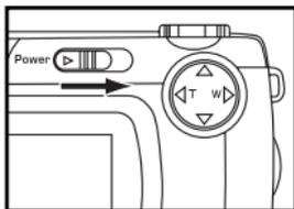
**1 Rotate the function dial to
