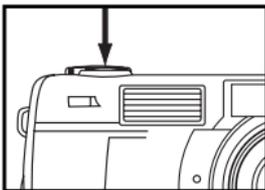
**8 Press and hold the shutter-release button all-the -way down.**
