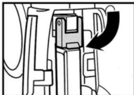
**3 Fold the card-release lever down as shown in the figure.**
