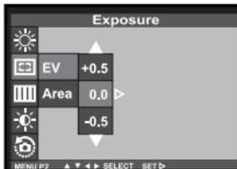
**4 Press the ▲ or ▼ key that the desired exposure compensation value appears ► to finish the setting.**
