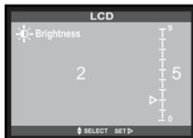
**3 Press the ▲ or ▼ key so that the desired brightness is highlighted. press ► will be set the value you changed.**
