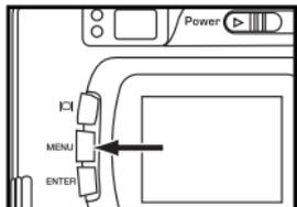
**1 Rotate the function dial to
