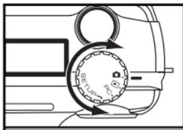
**2 Rotate the function dial to "SETUP".**
