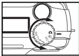
**2 Rotate the function dial to "SETUP".**
