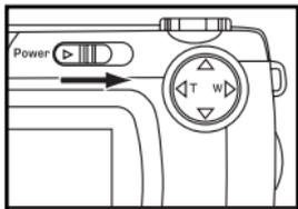
**2 Slide the power switch to turn on the camera.**
