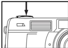
**7 Press the shutter-release button part-way down.**
