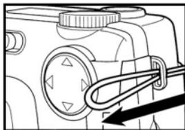
**1** Insert the smaller loop of the hand strap through the strap eyelet.
