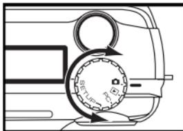
**1 Rotate the function dial to ▼ and press the MENU button.**
