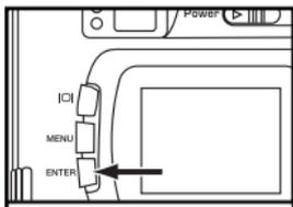
**9 To complete the operation of deleting an image, after confirming that [NO] is highlighted in the display to confirm, press the ► .**
