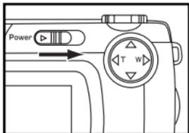
**1 Rotate the function dial to
