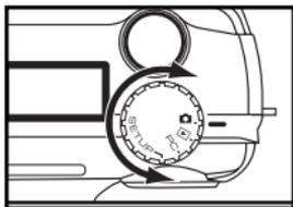
**2 Rotate the function dial to "SETUP".**
