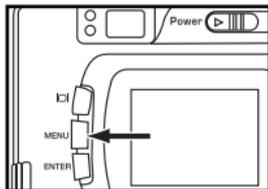
**1 Rotate the function dial to
