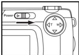
**1 Rotate the function dial to
