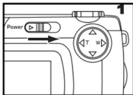
**1 Rotate the function dial to
