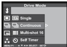
**3 Press the ▲ or ▼ key so that [Continuous] is highlighted and press ► key to finish the setting.**
