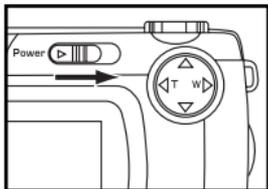
**1 Rotate the function dial to
