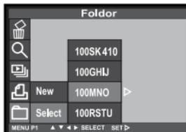
**5 Press the ▼ key so that the folder name in which the image to be played back is recorded is highlighted and press the ENTER button.**
