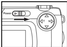
**1 Rotate the function dial to
