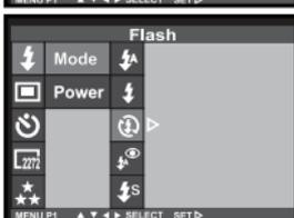
**4 Press the ▲ or ▼ key so that the desired flash mode in highlighted and press the ► key to finish the setting.**
