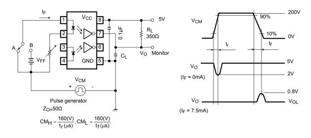
\* C<sub>L</sub> is approximately 15pF which includes probe and stray wirng capacitance.
