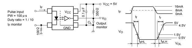
C<sub>L</sub> is approximately 15pF which includes probe and stray wiring capacitance.
