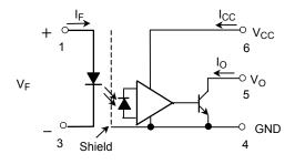
Note. A  $0.1\mu F$  bypass capacitor must be connected between pins 4 and 6.
