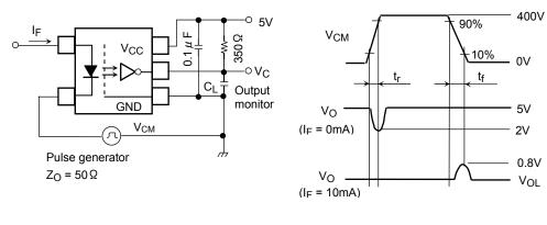
$$CM_{H}=\frac{320(V)}{t_{\Gamma}(\mu s)},CM_{L}=\frac{320(V)}{t_{f}(\mu s)}$$
