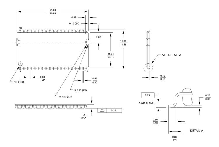
**NOTE:** 1. All dimensions in millimeters  $\frac{MAX}{MIN}$  or typical where noted.
