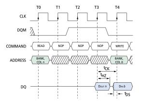
NOTE: A CAS latency of three is used for illustration. The READ command may be to any bank, and the WRITE command may be to any bank. If a burst of one is used, then DQM is not required.
