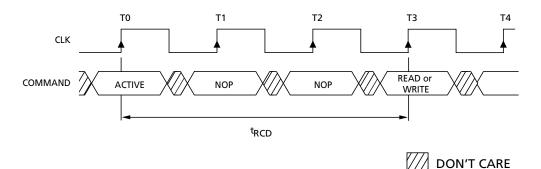
Figure 4 EXAMPLE: Meeting <sup>t</sup>RCD (MIN) when  $2 < {}^{t}RCD$  (MIN)/<sup>t</sup>CK  $\leq 3$
