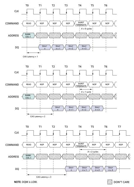
Figure 12 Terminating a READ Burst
