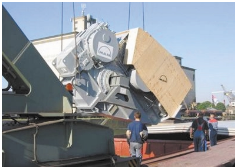
Takraf SRs 4000 – Transport of 2 x 1,000 kW bucket wheel gearbox for the Bulgarian installation.
