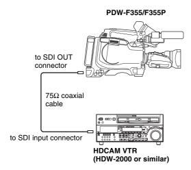
You can perform digital dubbing by connecting the SDI OUT connector of this unit to an external device with an SDI input connector.
