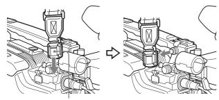
Pull in the direction of the arrow while pressing here.
