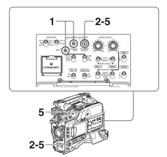
With the SUB CLIP indicator off, hold down the SHIFT button and press the THUMBNAIL button.
