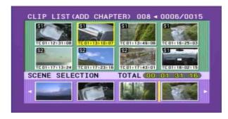
**3** Using the SEL/SET button or MENU knob, from the positions of the essence marks recorded within this clip, select the chapter for the part you want to include in the clip list. To select two or more chapters, hold down the SHIFT button and operate the MENU knob.
