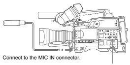
AUDIO IN (CH-1/CH-2) switches Set the AUDIO IN switch for the channel on which you want to record the audio to FRONT (for CH-1/ CH-2) or F (for CH-3/CH-4).
