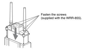
4 Engage the V-shaped plate on the back of the CA-WR855 with the V-groove on the battery attachment shoe, and then slide the CA-WR855 down until it connects to the WRR connector.
