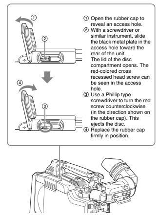
After removing the disc, it is not necessary to return the screw to its original position. When the power supply is restored, the mechanism will again function normally.
