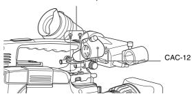
**3** Open the CAC-12 and remove the microphone adaptor.
