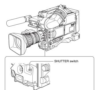
The current shutter setting indication appears for about 3 seconds in the setting change and adjustment progress message display area of the viewfinder screen.
