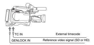
Example 2: Connecting two units, and using one as the reference
