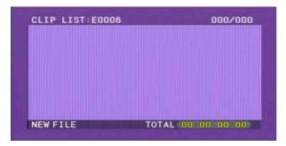
4 Hold down the SHIFT button, and press the SEL/SET button down (CLIP MENU).
