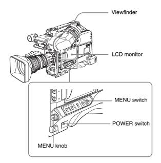
When the camcorder is powered on, flick the MENU switch to the ON position to display the menu on the viewfinder screen and the LCD monitor.
