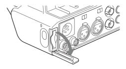
2 Insert the "Memory Stick" with its label side facing the "Memory Stick" logo on the camcorder.
