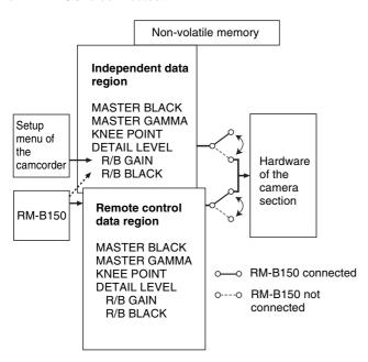
Thus, when a remote control unit is connected to the camcorder, the effective data region is switched to the "remote control data region" and the settings of the paint adjustment that were in effect the last time the remote control unit was used are recalled.
