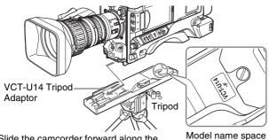
Slide the camcorder forward along the slot, until it clicks firmly into place.
