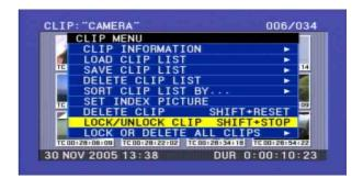
4 Use the SEL/SET button or MENU knob to select "LOCK/UNLOCK CLIP", and then press the button or knob.
