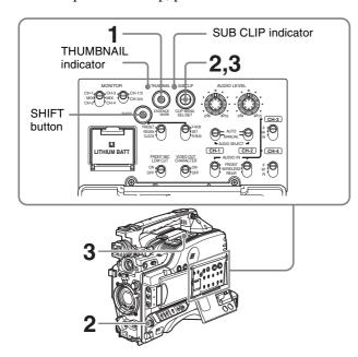
**1** With the SUB CLIP indicator off, press the THUMBNAIL button to turn the THUMBNAIL indicator on.
