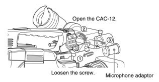
**4** Place an external microphone (electret condenser microphone such as the ECM-673/674/678) in the CAC-12.
