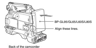
Slide the battery pack down until its "LOCK" arrow points at the matching line on the camcorder.
