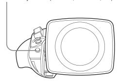
Remove the rubber cap on the front of the lens drive unit to reveal the iris sensitivity trimmer. Use a miniscrewdriver to turn the trimmer. Turn it clockwise to increase the sensitivity, and turn it counterclockwise to decrease the sensitivity.
