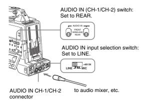
**2** Set the AUDIO IN input selection switch to LINE for the channel to which the external audio equipment is connected.
