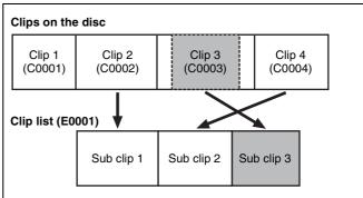
In the above example, the whole of clip 2 has been added as sub clip 1, and the whole of clip 4 has been added as sub clip 2. Sub clip 3 is part of clip 3. Therefore, when clip list E0001 is played back, clip 4 is played after clip 2, and then the part of clip 3 shown in gray color is played.
