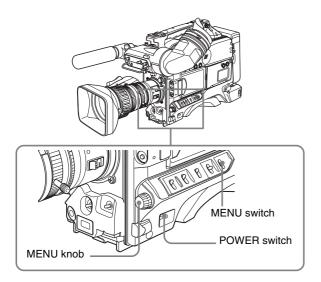
**1** Set the POWER switch to the ON position.
