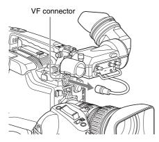
2 Loosen the viewfinder left-to-right positioning ring ①, and with the stopper raised ②, detach the viewfinder ③.
