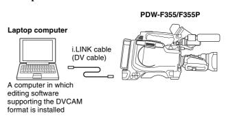
Operate the computer to set up the nonlinear editing software.
