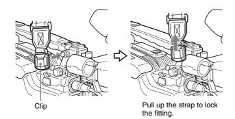
Fit the other clip to the shoulder strap fitting on the other side of the grip in the same way as in step 1.
