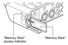
Insert a "Memory Stick". The "Memory Stick" access indicator lights up when the "Memory Stick" is being accessed for reading or writing.
