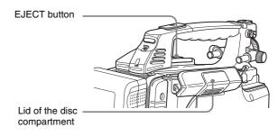
3 Insert the disc in the ▼ direction, and close the disc compartment lid manually.
